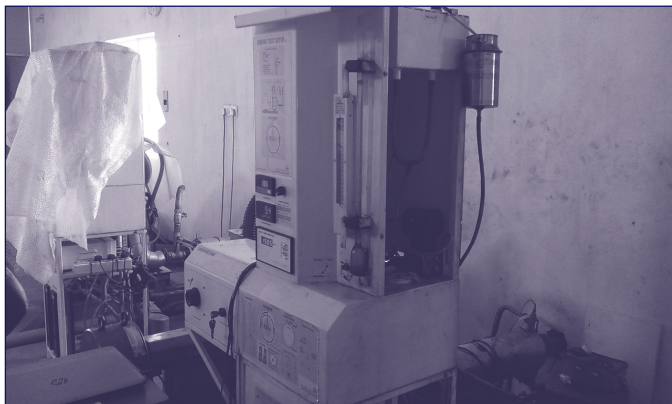
Figure 1: TV1 Variable Compression Ratio (VCR) Engine.
